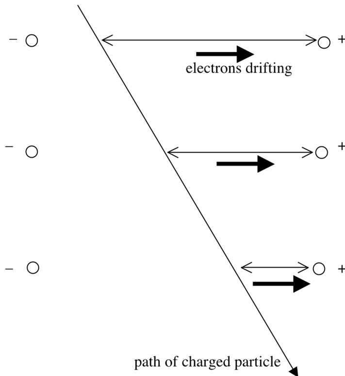
A charged particle enters the chamber along the path shown. Assume for simplicity that the path is along the plane of the page.
